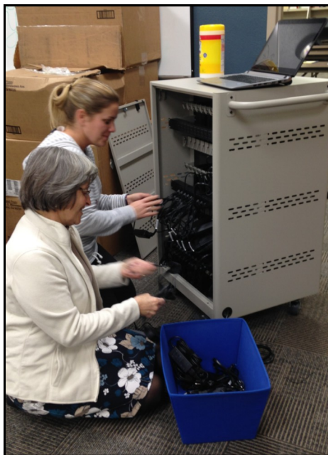
All 30 cords hang neatly in the back and plug into a power strip that draws from one heavy duty cord out of the ChromeCart.
